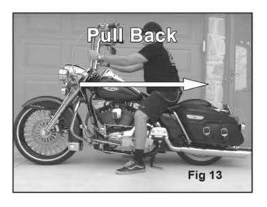
Note: If the center stand is difficult to operate and / or excessive force is needed to deploy the stand, something is wrong. Please review the usage instructions, videos, or contact Wheeldock if you have any concerns. Using excessive force will bend the lever arm. Bent lever arms are not covered under warranty.
